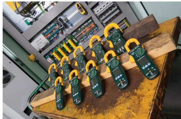
One of the convenient many uses for these meters includes troubleshooting fire alarm system end-of-line resistors as the meters will measure up to 60kΩ, which is grate than the value of the system.
