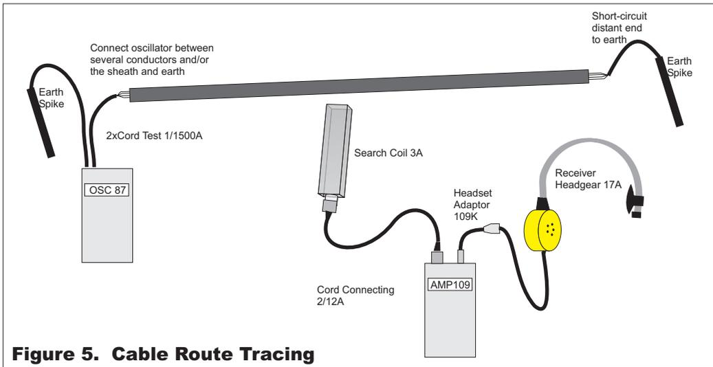
**Figure 5. Cable Route Tracing**
