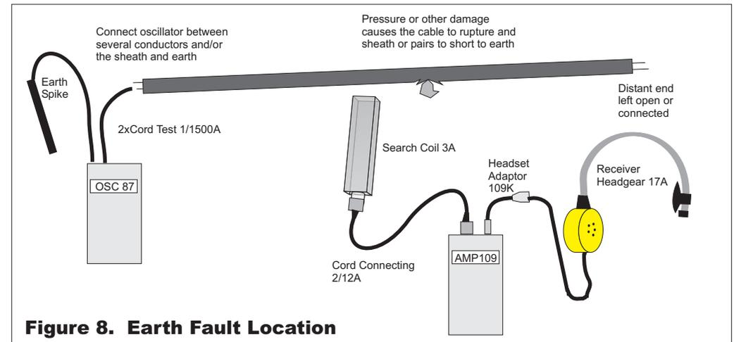
Figure 8. Earth Fault Location
