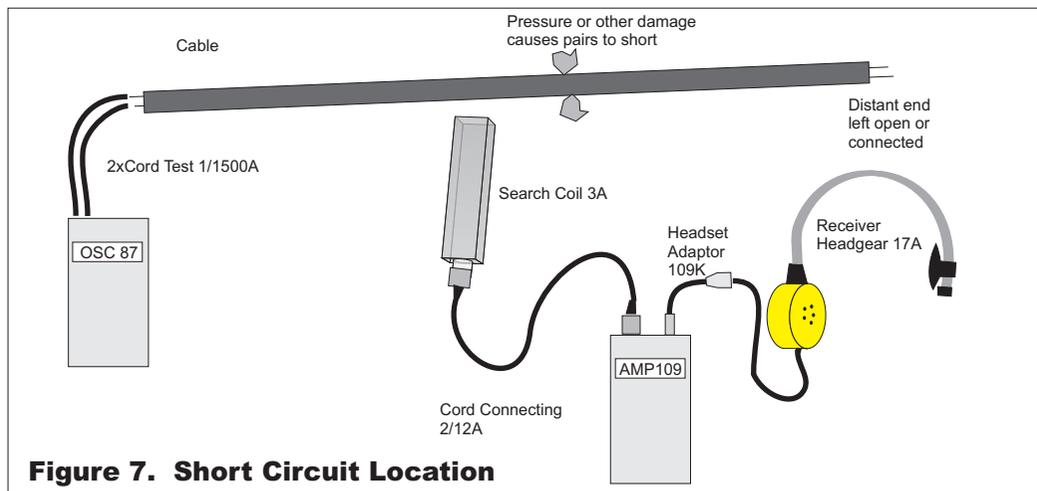
**Figure 7. Short Circuit Location**
