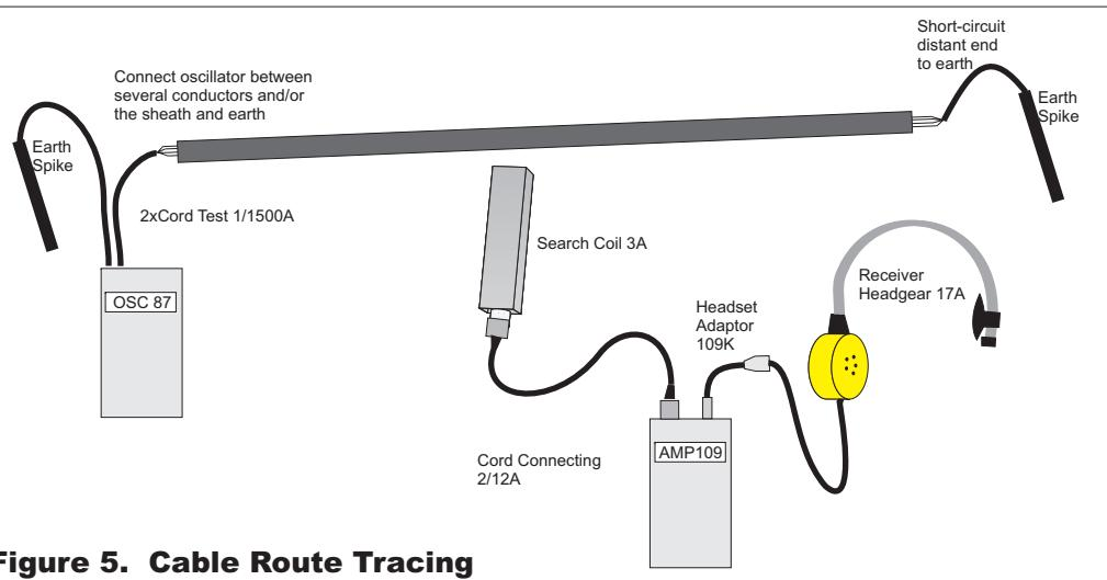
**Figure 5. Cable Route Tracing**
