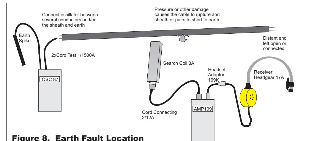
Figure 8. Earth Fault Location
