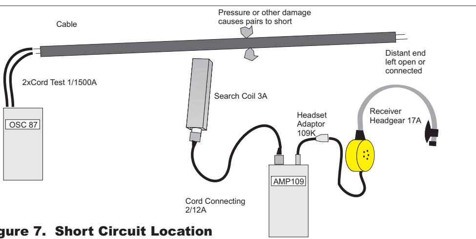
**Figure 7. Short Circuit Location**
